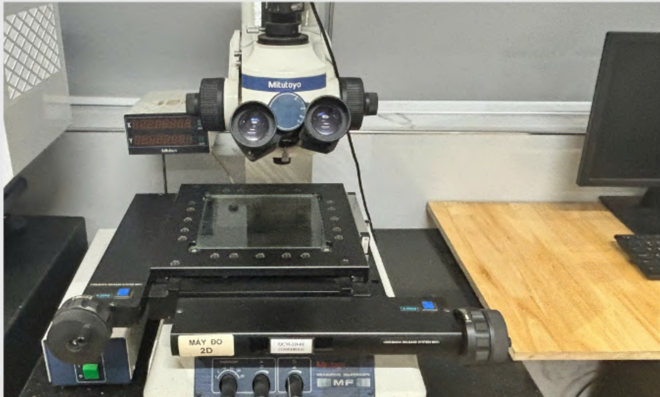
2D MEASURING MACHINE - MITUTOYO
